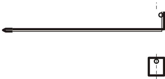
Fig. 2 — The bracket, drawn from the part drawing. Side elevation above, wall plate seen face on below.
